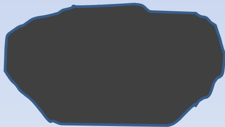
coating ball formed in the burning zone Soaked in the liquid for a long time. Hard and black, even in the core
