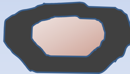
Snow ball formed in the transition zone Such balls normally melts in burning zone.The Core Is brownish
